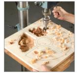
Rough out the interior using a drill press and a 2" Forstner bit.
