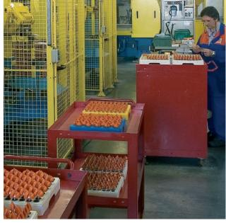
Loading the automated multi-axis CNC sharpening machines.
