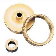
Beautiful, professional-quality inlays aren't as difficult as they seem. In fact, they're easy with a CMT Inlay Kit. Solid brass components come with either a solid carbide spiral bit or straight bit with 1/8" cutting diameter and 1/4" shank. Just remove and reassemble the small bushing to make the recess in the workpiece and cut out the inlay. Perfect for toymaking, puzzle making, lettering and lots of other decorative projects.
