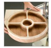
Bandsaw the exterior to final shape.
