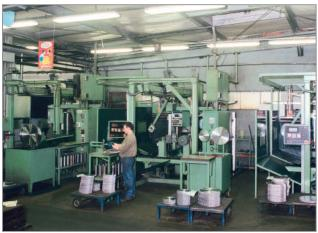
Grinding and tensioning the blades.
