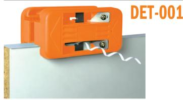
Attach this trimmer to your workpiece, press both ends against the board for a cutting range between  $13\text{mm}\ (1/2")$  and  $25\text{mm}\ (1")$ , move the trimmer in the correct direction indicated by the arrow. This will cut on both sides easily. The first cutter will cut straight, the second one can be adjusted for a tapering cut. Both cutters are made from high-quality hardened steel and can be easily replaced when worn out.
