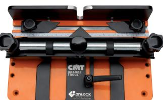
Clamp extension arm to make Edge-to-Edge joints.
