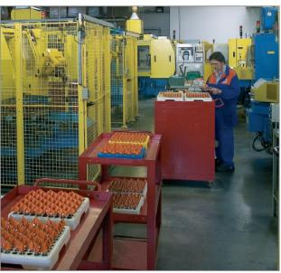
Loading the automated multi-axis CNC sharpening machines.
