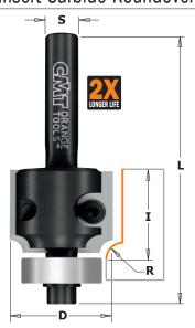
Roundover bits with two replaceable knives fixed by special Torx screws. The blades are profiled on 4 sides providing greater efficiency and precision when working on laminates. Small radius available 3/64", 1/16" and 1/8". For use on portable Routers.
