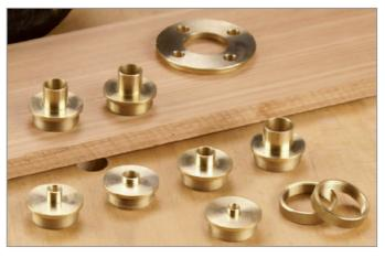
A practical 7-bushing kit that will extend the possibilities of your router. For template-controlled operations such as dovetailing, stair routing, hinge butt routing, lock face routing and more general template tasks. These template guides can be used with any router featuring a 30mm (1-3-/16") bore baseplate. Fits the most popular routers. Some routers require CMT's base 899.000.02.
